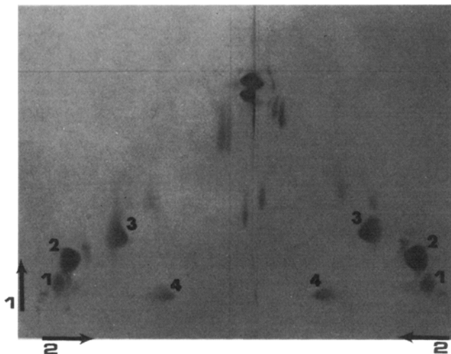
FIG. 1. 2D-TLC of 2 crude soybean lipid samples on one TLC plate. Origins are lower left- and right-hand corners. Basic solvent (#1), chloroform/methanol/7N NH 4 OH, 65:30:4, from bottom to top. Acidic solvent (#2), chloroform/methanol/acetic acid/water, 170:25:25:4, from right to left and after drying, from left to right. Spots are identified as 1: phosphatidylinositol; 2: phosphatidylcholine; 3: phosphatidylethanolamine; 4: phosphatidic acid. Sunflower phospholipids migrated in the same way and plates were identical to the one shown.
